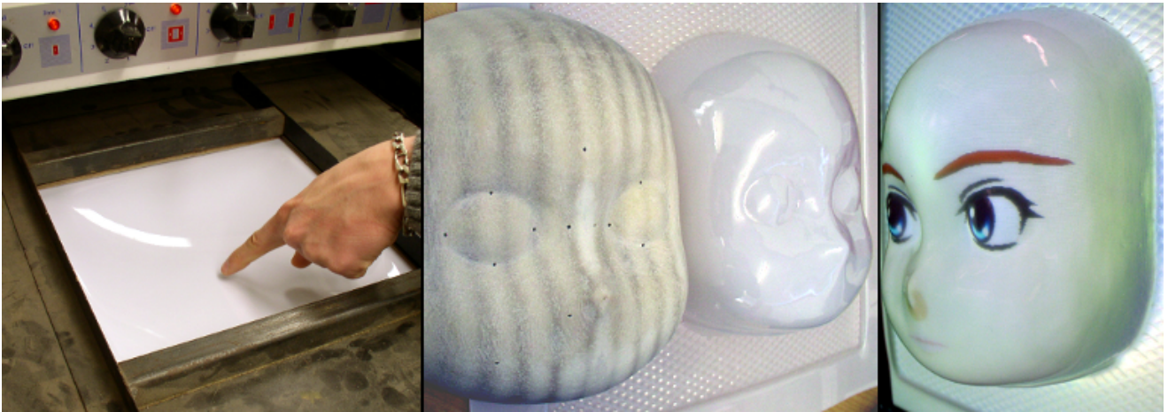
Fig. 4. Different stages of the process. Left: vacuum forming, middle: the mold and the resulting facial mask, right: an animated face is retro-projected into the facial mask.
