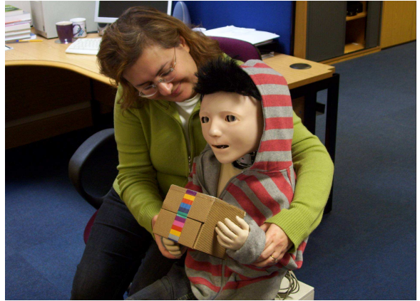
Fig. 1. Learning via Social Interaction. The humanoid robot Kaspar2 is taught how to hold a patterned box.
