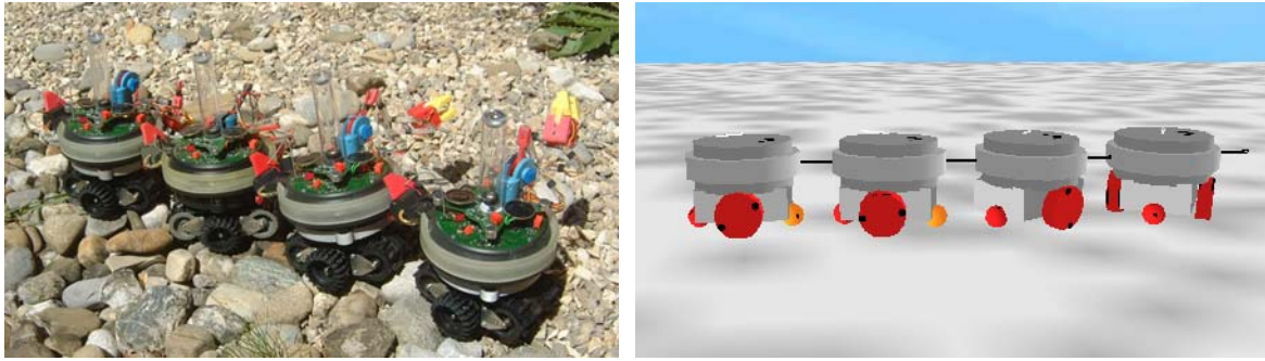
Figure 7. Left: Four robots assembled into a linear structure. Right: A simulation of the robots shown in the left part of the figure.
