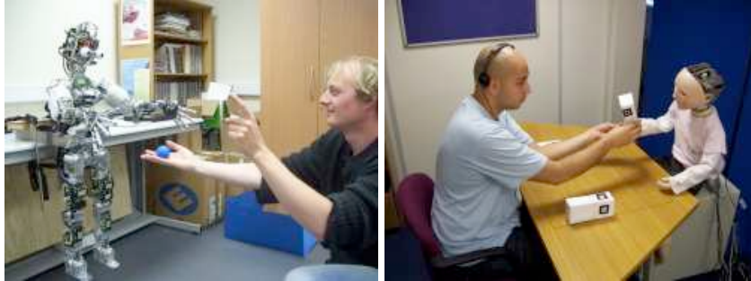
Fig. 1. Humanoids iCub (left) and Kaspar (right) used in language acquisition studies. These studies include work on learning vocabulary, holophrases, negation and grammar in a manner where language is grounded in active manipulation of objects, the social environment, and in sensorimotor experience in unconstrained interaction with human teachers. The work is targeted at the acquisition of human language-like capabilities.
