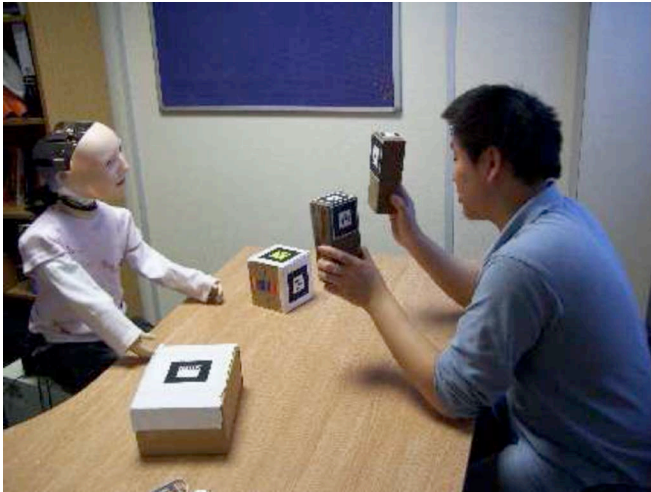
Fig. 1. The humanoid robot Kaspar II, analogous to a young child, working with a teacher.
