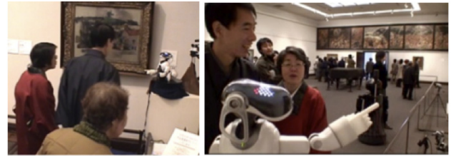
Fig. 1a and b: Sony AIBO used as a museum guide robot. In order to make the robot’s deictic gestures distinct, we attached a pointing shaped hand to the robot’s right arm.
