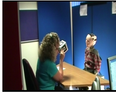
Fig. 1. Part of a session in the study with the humanoid robot Kaspar [2]. The participant was asked over five 2-minute sessions with the robot to explain the shapes on the box as if the robot were a small child. From session 2 onwards the robot responded to the presented shapes by querying its association between salient words spoken by the participant in the previous session with its sensorimotor history and expressed a chosen word.
