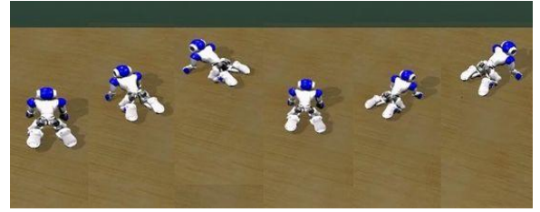
Fig. 8. NAO crawling and turning behaviours. The left three graphs show crawling left with Al = 0.15 , Ar = 0.25 , |Al - Ar| = 0.1 . The right three graphs show crawling right with Al = 0.25 , Ar = 0.18 , |Al - Ar| = 0.07 . The degree of turning left is greater than turning right.
