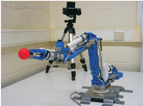
Figure 2: The setup consists of a 6 DOF arm and a stereo camera for respectively performing and perceiving actions.
