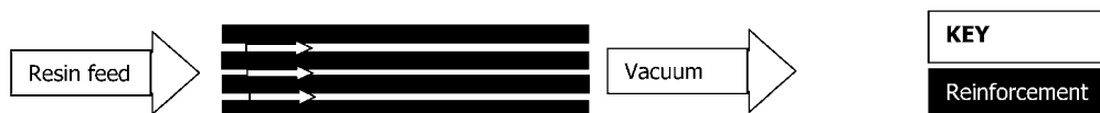
Fig. 1 Schematic representation of the resin infusion in-plane flow process [the bagging film (above) and mould tool (below) are omitted for clarity]
