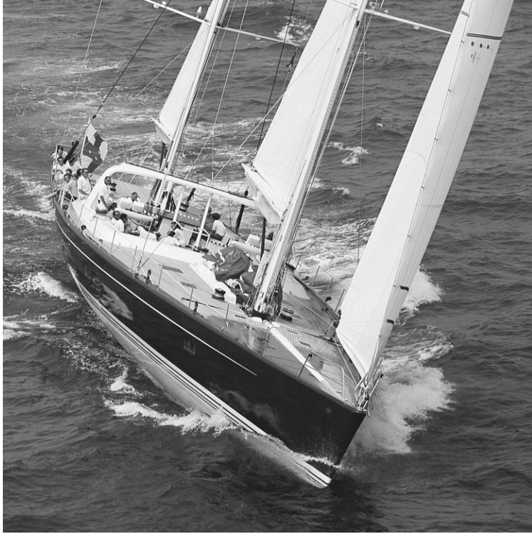
Figure 6 100' cruising yacht built using SP Ampreg 26 epoxy laminating resin, impregnated with a nip-roller wet-out machine and consolidated under a vacuum bag.
