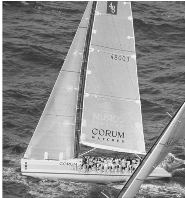
Figure 10 O/D 48' racing yacht built using SP Prime 20 epoxy infusion system and the SCRIMP process at TPI.
