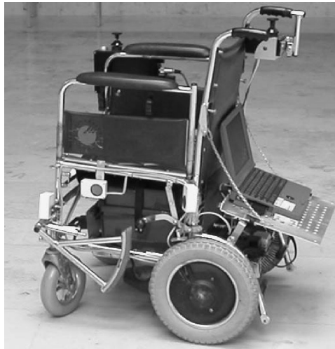
Figure 1 Wheelchair controlled by a laptop Pentium PC 133 MHz running the neural network simulation software, CORTEX-PRO. Sonar sensors in small white boxes are used to avoid collisions and for self-localisation
