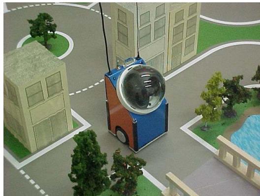
**Figure 1.** Experimental set-up. A miniature remote-brained robot with a 8cm x 8cm base performs vision-guided navigation in a 170 cm x 120 cm model town, following a sequence of actions defined in prior instructions given by a user. Video images are sent by wireless from the robot to a PC for processing. The resulting motion commands are sent back by wireless to the robot. The user speaks to the robot through a headset microphone connected to the PC.
