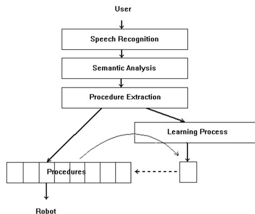
**Figure 2.** IBL concept diagram. A command issued by the user can either be executed immediately if the robot has the corresponding procedure, or a learning process is initiated. Thereby, a new procedure is created from a combination of existing primitives.
