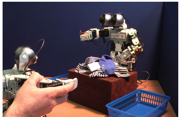
Fig. 1. Experimental setup for investigating grasping locations on an item of clothing from a pile of randomly positioned clothes. In the foreground a similar Bioloid robot is used to remotely control the other.
