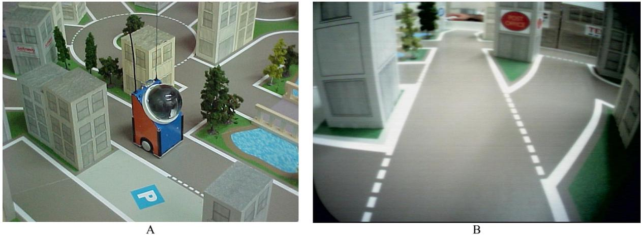
**Figure 6** *A. Miniature robot (base 8cm x 8cm). B. View from the on-board colour camera*
