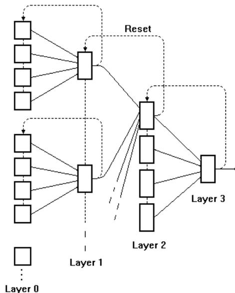
Figure 1: Architecture of the neural network used to model a subset of active neurons in the visual system. The pyramidal network has 64 neurons in its input layer (Layer 0), divided in 16 groups of 4 neurons connected to 16 neurons in layer 1. These neurons are divided into 4 groups of 4 neurons connected to 4 neurons in layer 2. These 4 neurons are connected to a single neuron in layer 3.
