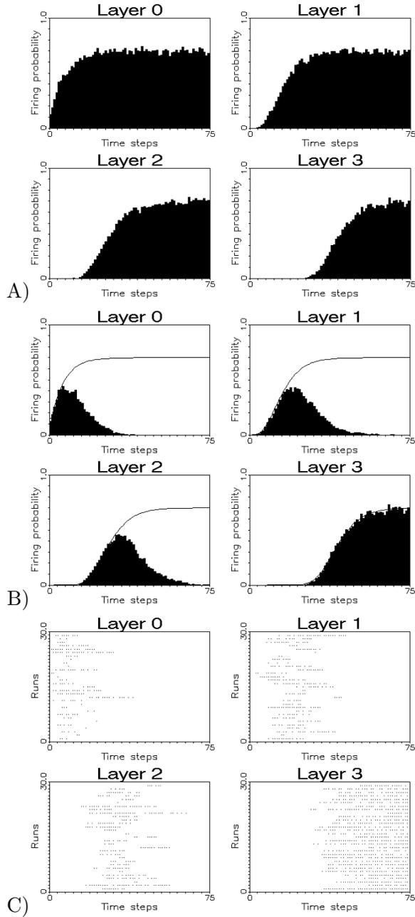
Figure 2: A) Temporal evolution of the firing probability in the case without reset by the inhibitory feedback. B) Same as A) with reset. C) Spike raster of 30 runs in the case with reset. Each dot indicates the time of occurrence of a spike. Simulation parameters:  $p_0 = 0.15$ ,  $p_1 = 0.7$ . Histograms are based on 500 runs. The continuous line in B) is the theoretical prediction given by equation (17).
