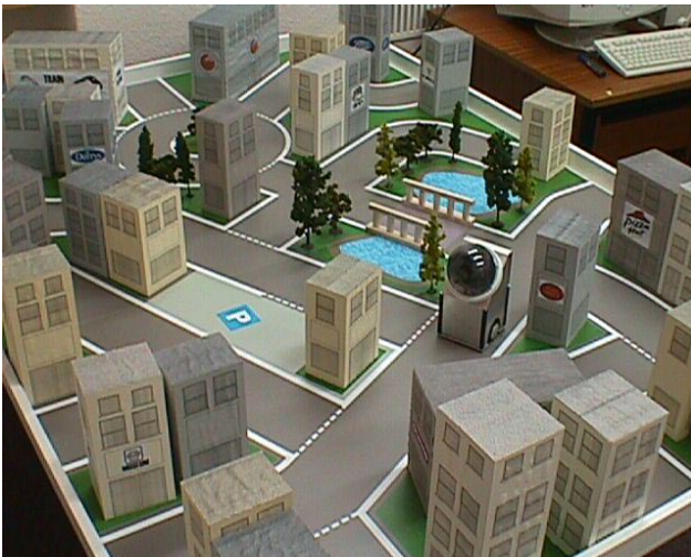
Figure 1. Experimental set-up. A miniature remote-brained robot performs vision-guided navigation in a model town, following a sequence of actions defined in prior instructions given by a user. Video images are sent by wireless from the robot to a PC for processing. The resulting motion commands are sent back by wireless to the robot.
