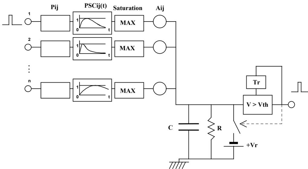
**Figure 1.** Extended Leaky Integrate-and-Fire neuron. The features are explained in the section 2. The simulation results shown in the paper are obtained on a PC with the simulation package CORTEX-PRO.
